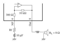
Bass boost can be easily implemented by inserting a series connection of RC between Pin8 (output) and Pin6 (NF). Example :  $Rb = 12 k\Omega$ ,  $Cb = 0.022 \mu F$
